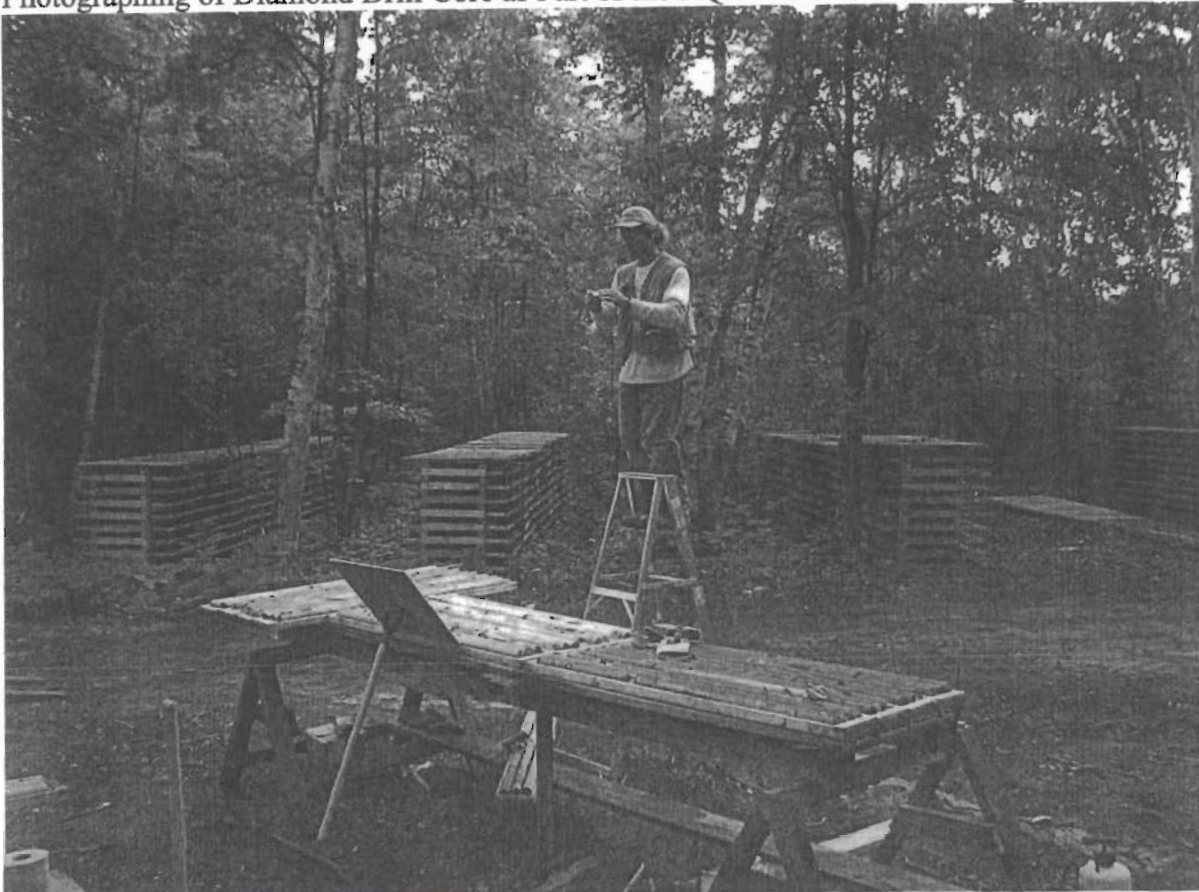
Photograph: 8.0 Douglas MacMillan, B.Sc., Geo. taking digital photographs of NQ core from diamond drill hole U-03-60, as part of the process during the collection of the diamond drill hole RQD data collection.
