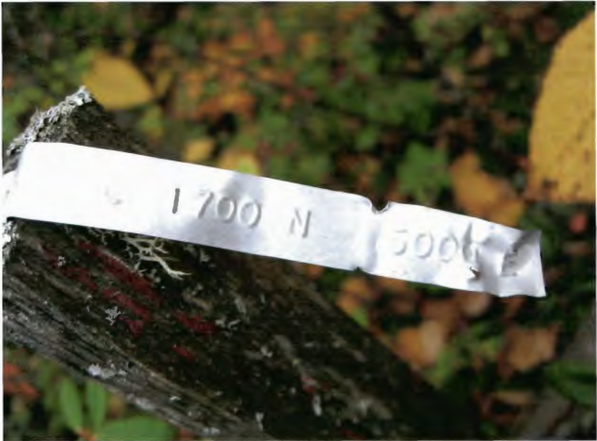
Figure 26. Small (once red) picket from Pick Lake grid – DYMO tag still legible and attached.
