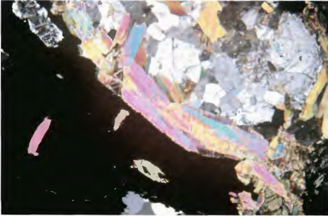
PLATE 23 PLB C-1: Birefringent red-yellow mica in quartzofeldspathic fragment with hornblende, same field of view as Plate 21 crossed polars.
