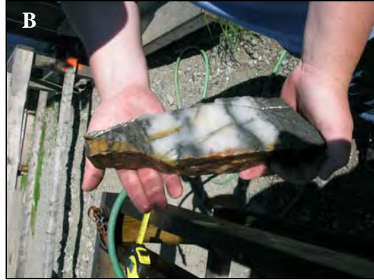
Photograph of: A- shear zone with quartz vein as it outcrops of the B4-16 anomaly. And, B- fresh cut surface of channel sample across main quartz vein showing wall rock inclusions with seams of sulphide up to 12%
