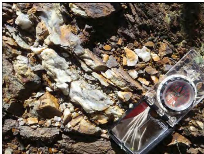
Photograph of quartz vein from B4-10 EM anomaly. Note visible seams of pyrrhotite with in bulk of vein.
