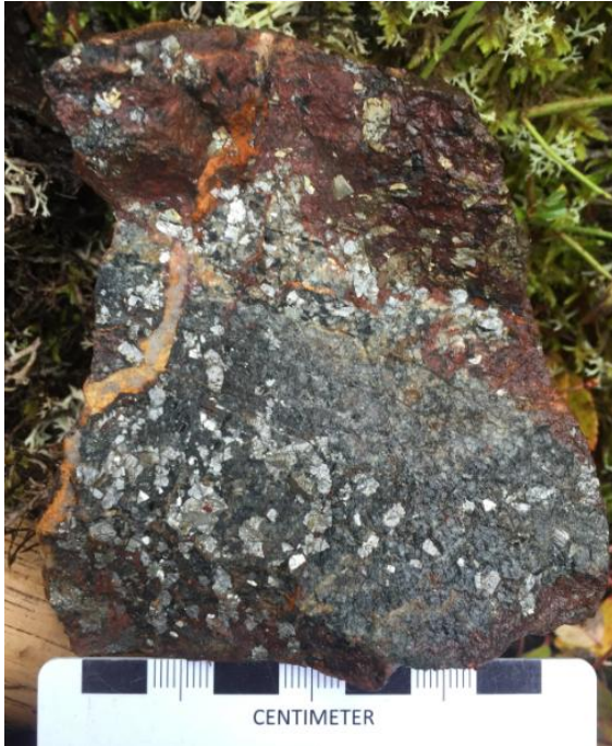
Figure 4 (Left). Mineralization style 1 from the Wiggle Creek Showing. Coarse-grained arsenopyrite is the dominant sulphide, disseminated in host proximal to discordant quartz/carbonate veins. Mineralization here is found in interbedded iron formation and metasediments.
