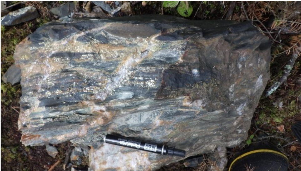
Figure 2. Mineralization style 1 from the L28 Showing (Target 3). Quartz veins discordant to banded iron formation with coarse pyrite mineralization concentrated in bedding parallel veins and fractures as well as disseminated in the host proximal to veins.
