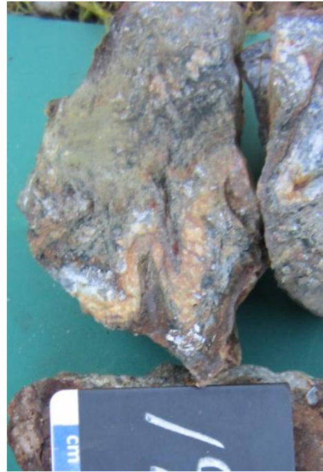
Figure 4 (Left). Mineralization style 1 from the Wiggle Creek Showing. Coarse-grained arsenopyrite is the dominant sulphide, disseminated in host proximal to discordant quartz/carbonate veins. Mineralization here is found in interbedded iron formation and metasediments.
