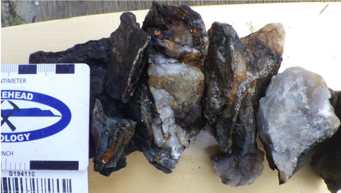
Figure #. Sample S194110. Example of mineralization style 4, 1 – 2 mm wide band of pyrite-rich massive sulphide with minor chalcocopyrite and pyrrhotite within chlorite altered sediment host.
