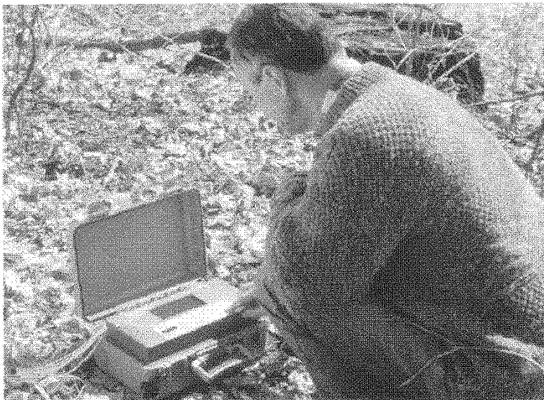
The IPR-12 Receiver measures up to eight dipoles simultaneously. It then records measured and calculated parameters in memory.
