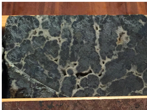
Figure 12: Chalcocite vein breccia from SB Zone drill hole BCP-19-11. Note drusy quartz-lined voids
