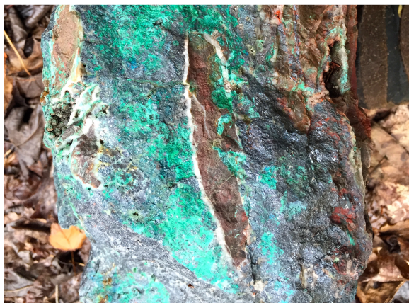
Figure 11: Chalcocite vein breccia from a B Zone trench. Note drusy quartz-lined voids.
