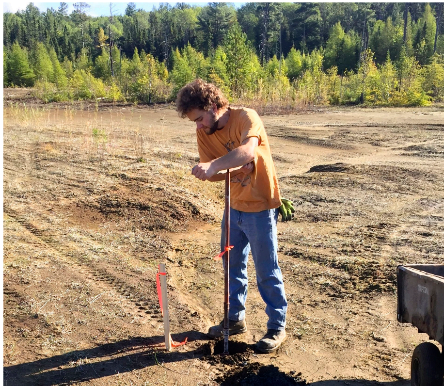
Photo 8.0 – Auger Sampling Kanichee Tailings Impoundment
