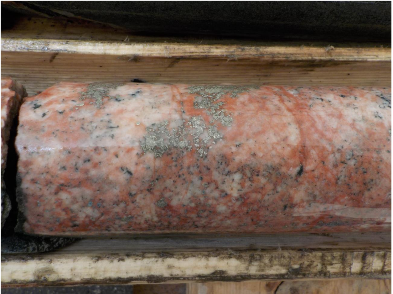
Close-up of strongly bleached diorite with pyrite
