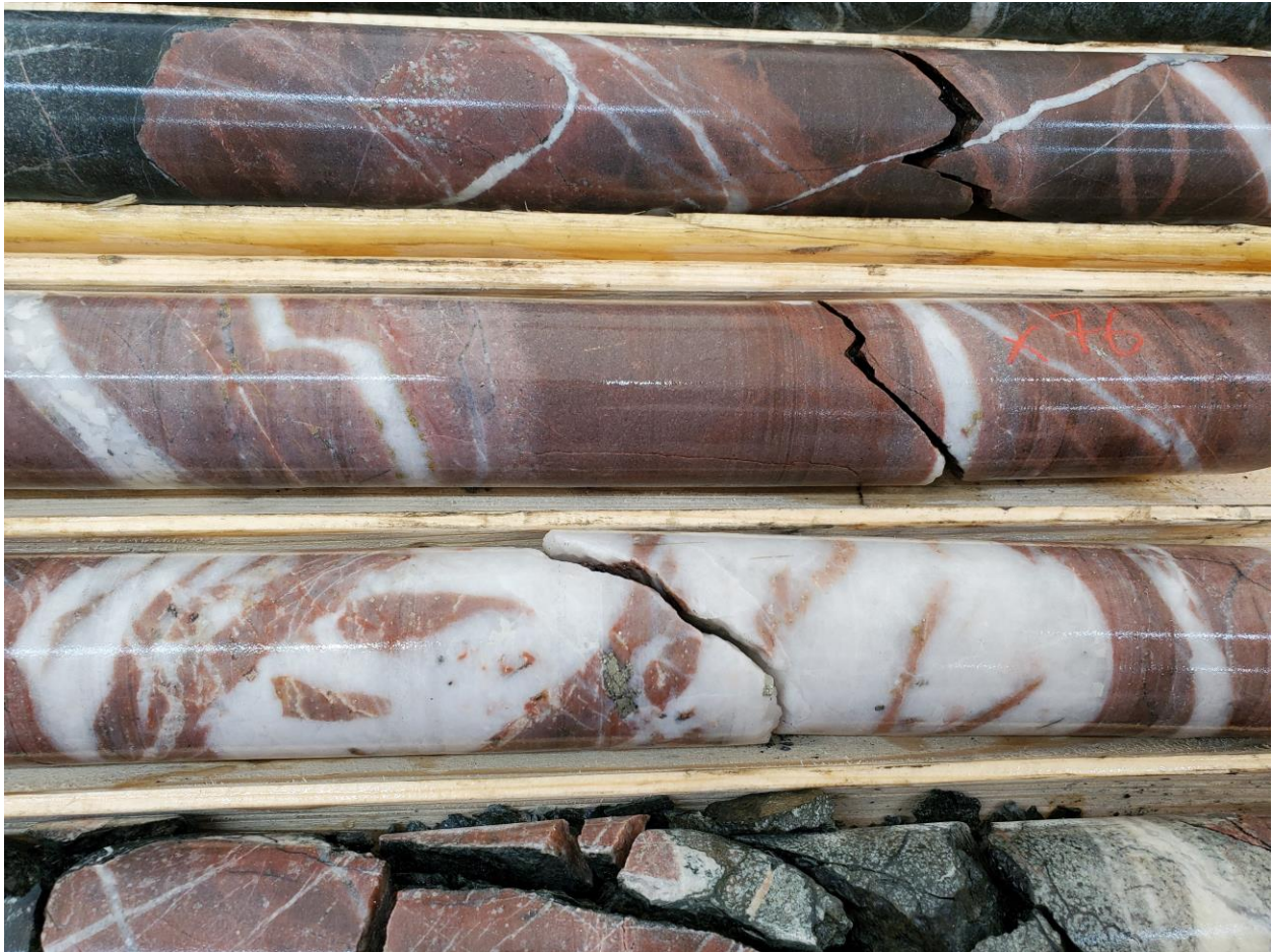
Close-up of alteration and veining in monzonite / monzodiorite dykes
