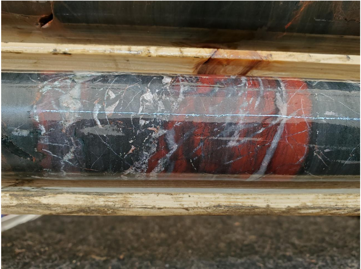
BIF with quartz stringers, pyrite in fractured hematite band
