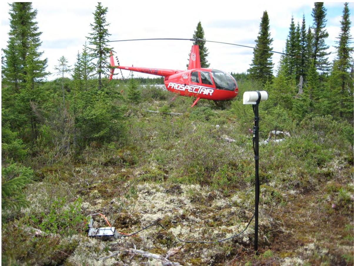
Figure 6: Example of a magnetic base station setup
