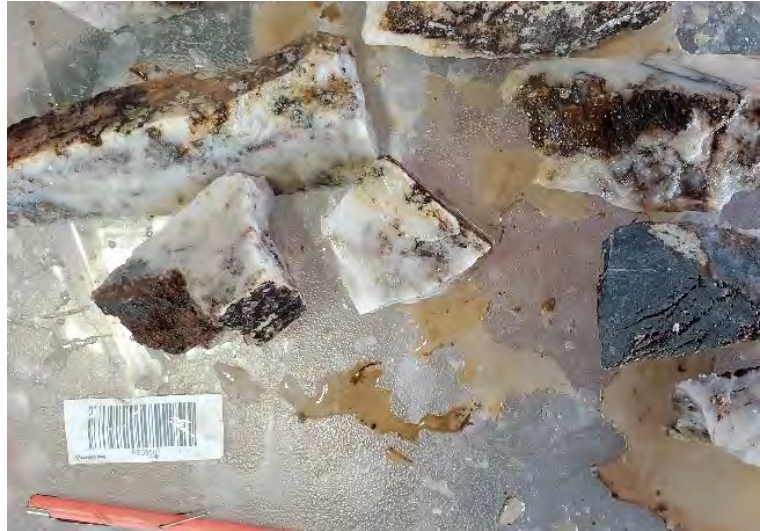
Figure 39. Channel sample F809507 (Moretti-Main North Vein prospect) returned 51.5 g/t Au and 1.38 g/t Ag over 1.0 m.
