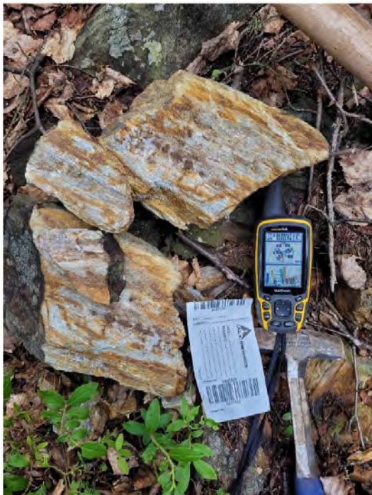
Figure 7-5 Sample S8597435 of sheared and mineralized granodiorite.
