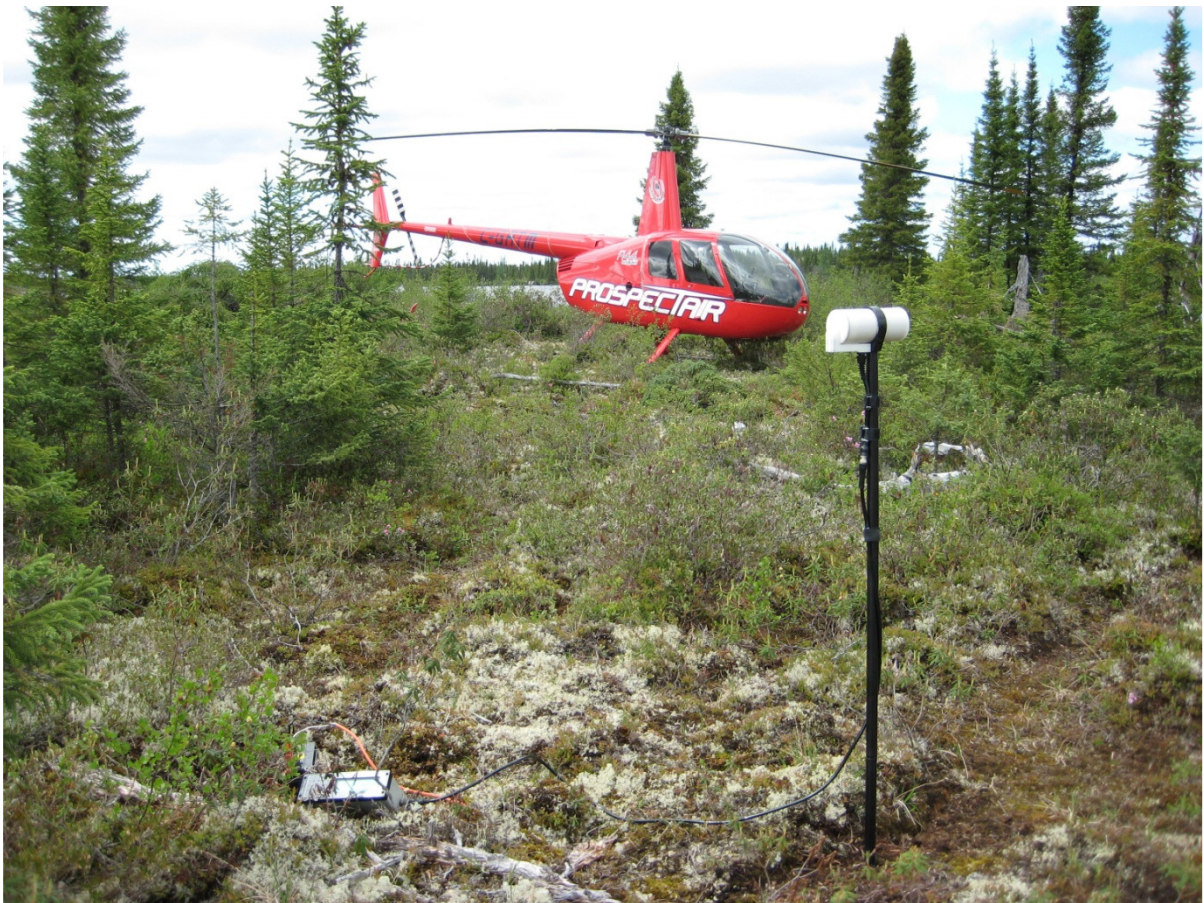
Figure 5: Example of a magnetic base station setup
