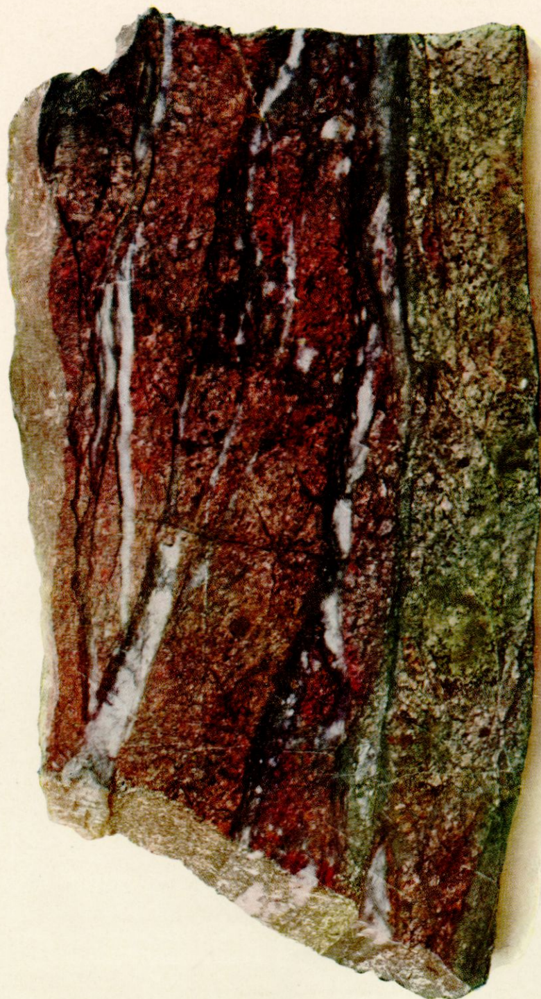
Polished Sample (natural size) of high-grade Gold Ore in Red Porphyry and Syenite, from Kirkland Lake mine. This ore is typical of the Kirkland Lake Area.
