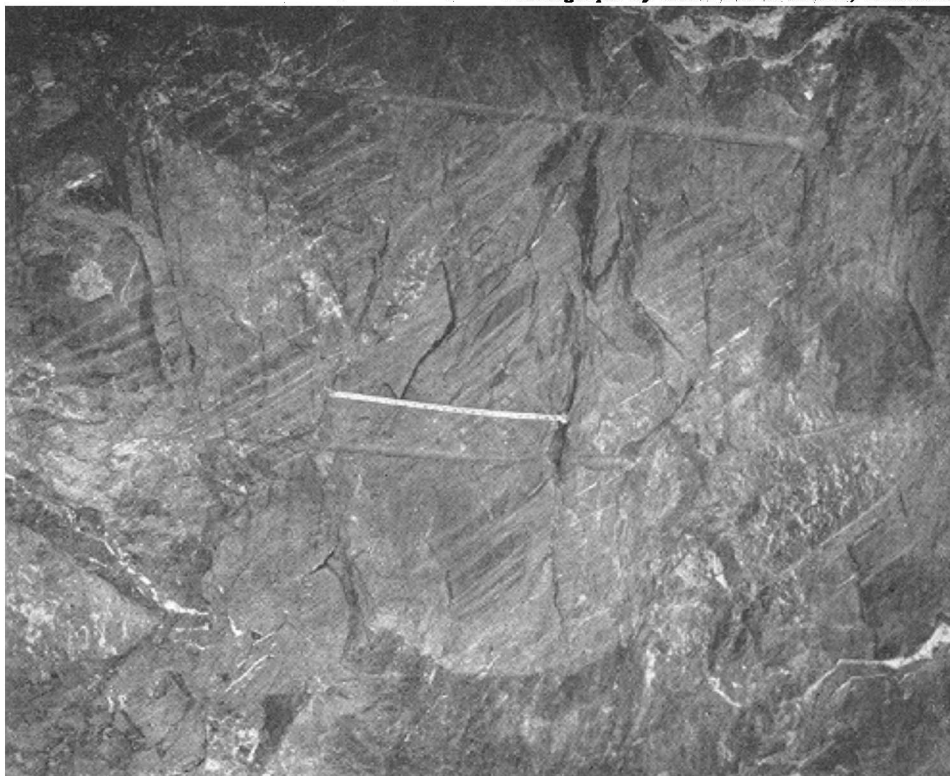
Jointing along the walls of a vein in syenite porphyry at the Lake Shore mine. Alteration has taken place along the set of joint planes.
