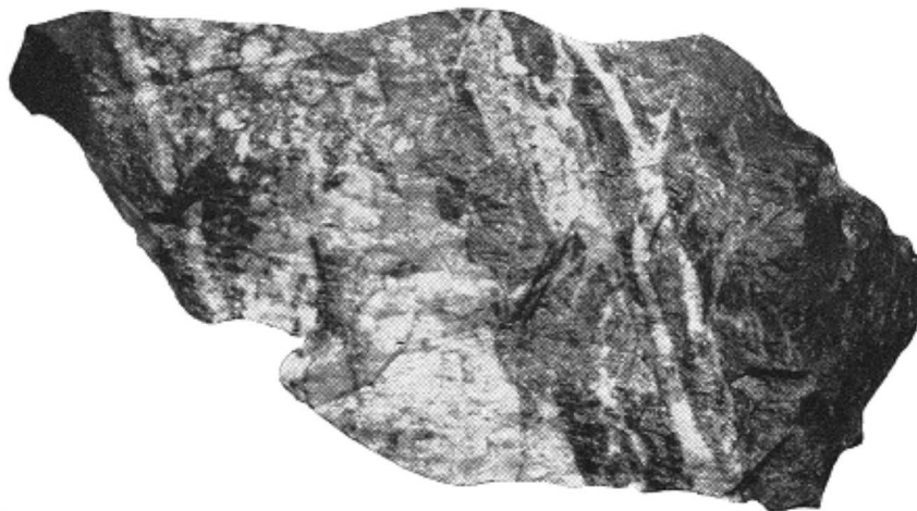
Specimen (one-quarter natural size) of gold ore in tuff from 4.D stope, 4,300-foot level, Kirkland Lake Gold mine.
