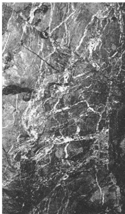
Vein breccia and quartz stockwork in tuffs, exposed on the back of No. 4601 east drift, Sylvanite mine.
