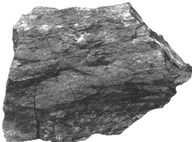
Specimen (one-half natural size) of mylonite from the main zone of displacement of the Kirkland Lake fault, 4,000-foot level, Wright-Hargreaves mine.
