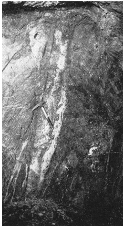
Exposure of the North vein on the 3,000-foot level, Wright-Hargreaves mine, showing the well-defined footwall (lower right corner). The wall rock is syenite porphyry.
