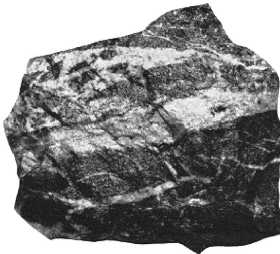
Specimen (one-quarter natural size) of high-grade ore in syenite porphyry from No. 1065 stope, 1,000-foot level, Sylvanite mine.
