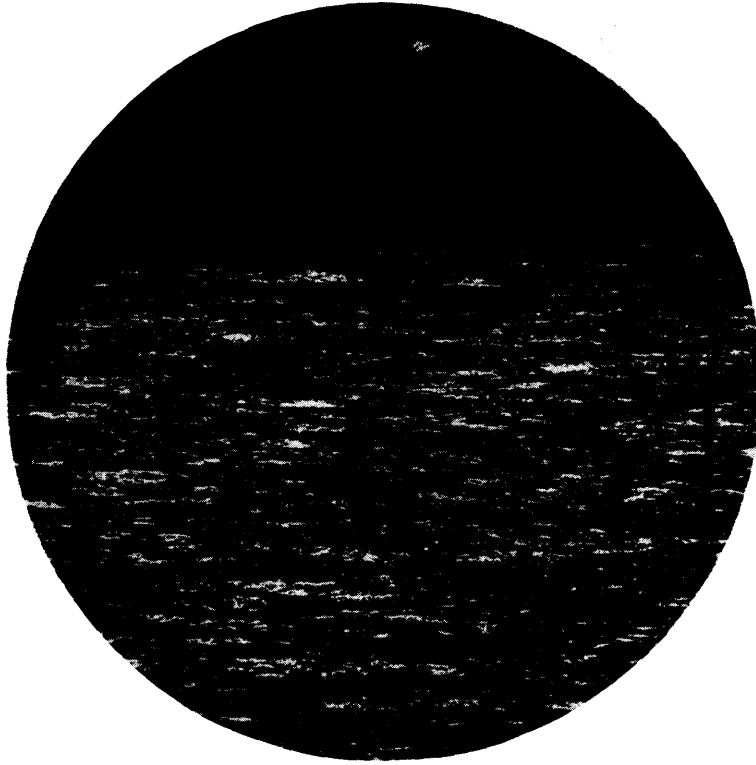
Fig. 12—Example of Straight Fatigue Magnification \times 100
