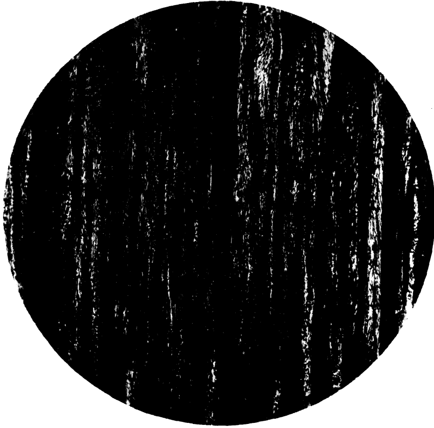
Figs. 8 and 9.—Effect of Cold Drawing on Lamellar Pearlite Magnification \times 1000
