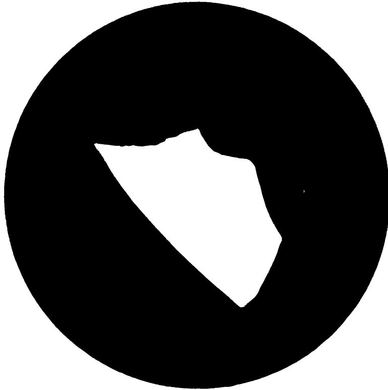
Fig. 35 (a)—Cross Section of Outer Wire Cut from Rope, 1250 ft. from skip. Loss of Metal = 22.3%
