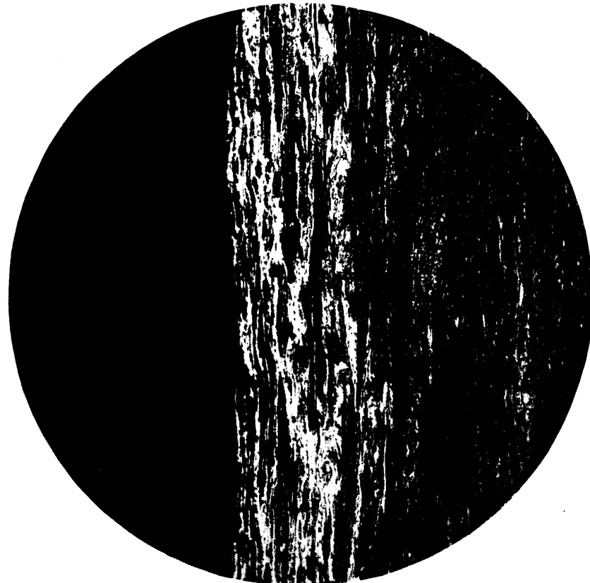
Fig. 10—Longitudinal view of edge of wire. Showing surface decarburization to depth of .004 inches Magnification \times 250
