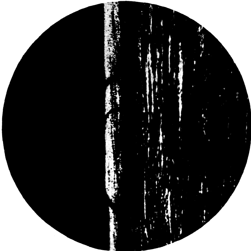
Fig. 22—Martensite on a Cage Rope from a Vertical Shaft. Service 1 month Magnification \times 1000
