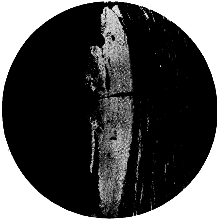
Fig. 17—Martensite on Hoisting Rope. It is some- times white etching and structureless. Magnification \times 500
