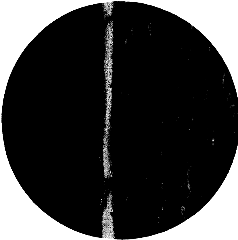
Fig. 19—Martensite on Skip Rope from an Inclined Shaft. Service 13 months Magnification \times 500
