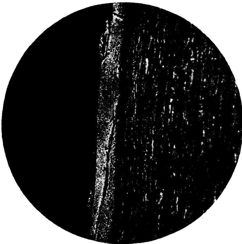
Fig. 20—Martensite on a Cage Rope from a Vertical Shaft. Service 21 months Magnification \times 500
