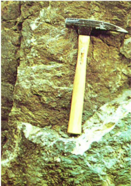
Photo 120. The east trench wall, Bi-Ore Mine, Cobre Lake. The vein comprises massive chalcopyrite (brassy) in quartz (grey) and carbonate (white). Weathering has developed malachite (green) and limonite (brown).
