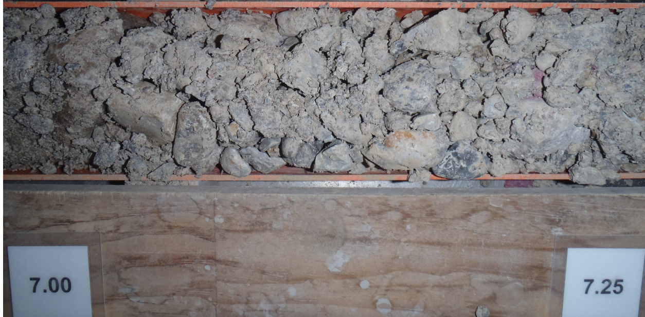
Photo 5. Typical pea- to cobble-size gravel bed within the Ypsilanti low-water phase deposits. Clast lithology is dominated by limestone and the matrix sediment is medium- to coarse-textured sand (Borehole LP-MW-01-10).
