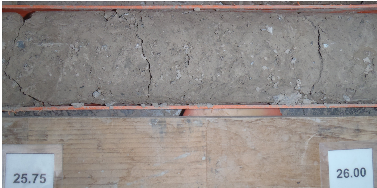
Photo 3. Borehole sample of Port Stanley Till: sandy silt to clayey silt diamicton with 10 to 15% grits to cobble gravel (Borehole LP-MW-01-10).
