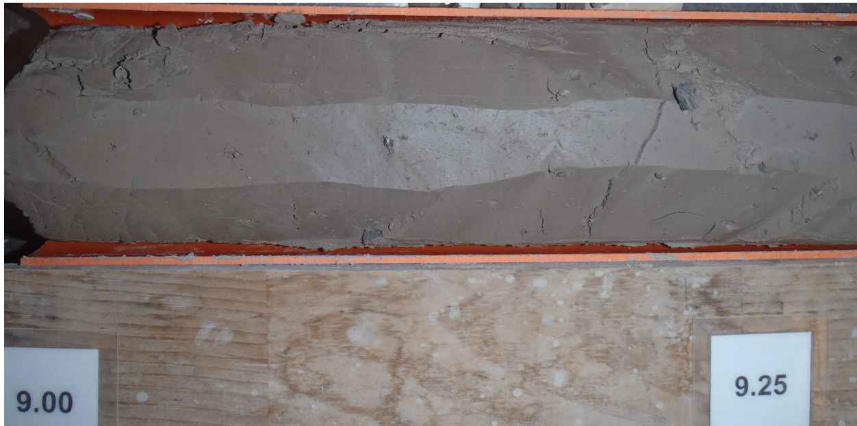
Photo 8. Borehole core sample of Wentworth Till. Massive, slightly sandy, clayey silt diamicton containing minor grits, granules and silt laminae (Borehole LP-MW-24-10).
