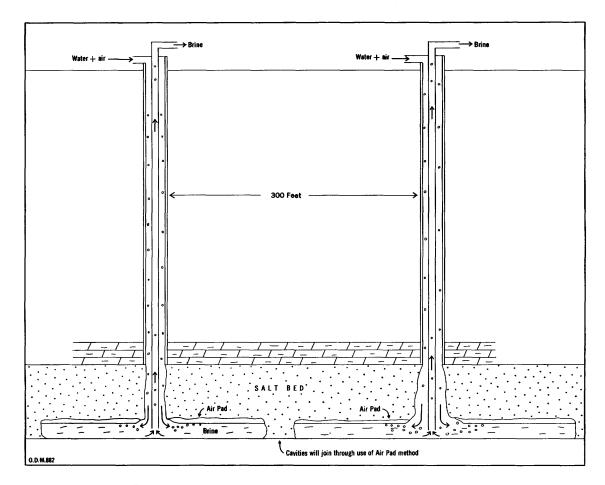
Figure 11 – Use of air pad method of joining two nearby wells.
