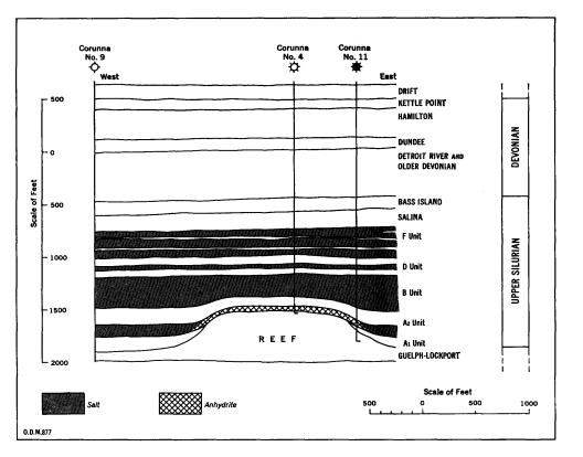
Figure 6 — Structure section showing nondeposition of A<sub>2</sub> salt, Corunna pool reef. (After R. O. Grieve.)
