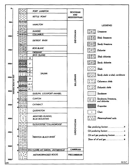
Figure 4 – Generalized columnar geological section for southwestern Ontario. (Courtesy Geological Survey of Canada)
