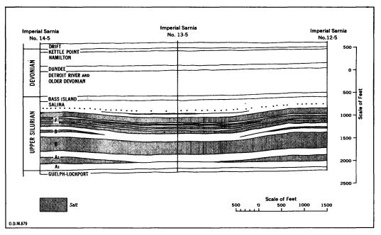
Figure 8 – Structure section showing removal of salt and subsidence, Sarnia area. (After R. O. Grieve.)
