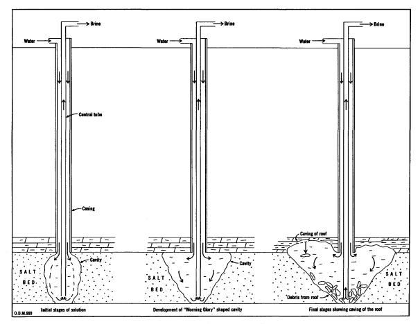
Figure 9 - Tully method of brine-well operation.
