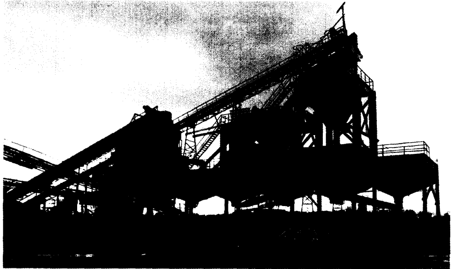
Photo NI-1-1. PROCESSING PLANT AT LINCOLN QUARRY SHOWING SYMONS CONE CRUSHER (LEFT), SCREENS AND BULK LOAD-OUT BINS.
