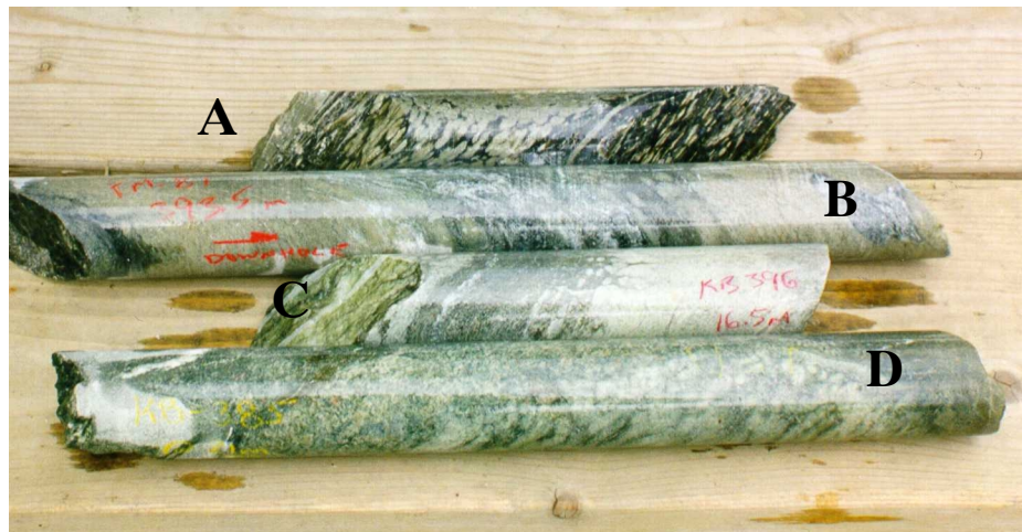
Photo 2. Diamond drill core intersecting variolitic mafic volcanic rocks from the collection of Pentland Firth Ventures Ltd. Samples from the Marhill Mine property (A and B, DDH PM-81), and the Bell Creek Mine property (C, DDH KB-396 and D, DDH KB385).
