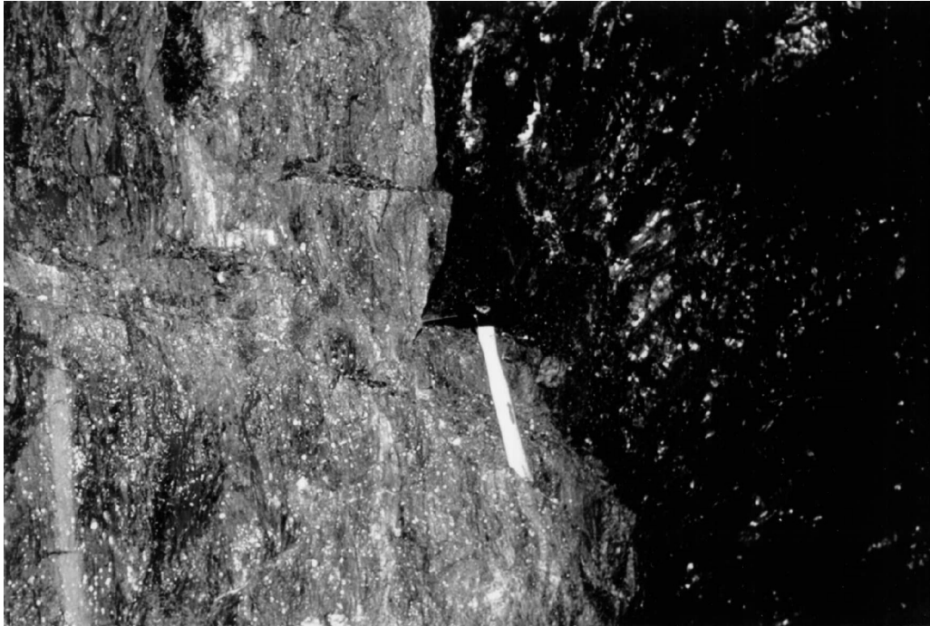
Photo 3. Contact between basalt (left) and graphitic argillite, Owl Creek East Zone, 725 crosscut south, looking west. Note presence of disseminated pyrite in basalt. Photo courtesy of Dan Brisbin.
