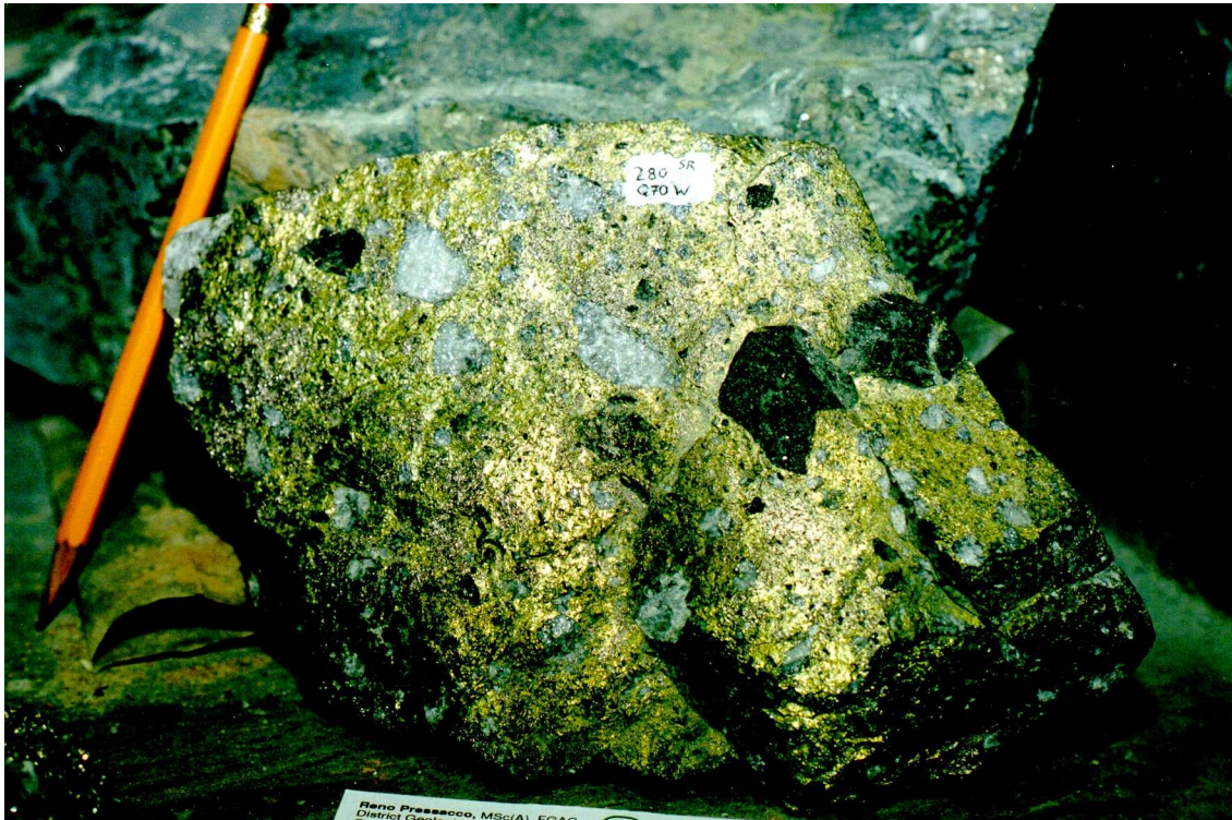
Photo 7. Hand sample of a cpy-rich sulphide breccia vein from the 280m level, Q70 Zone, Detour Lake Mine. Note the fragments of quartz and mafic wall rocks in a chalcopyrite matrix.
