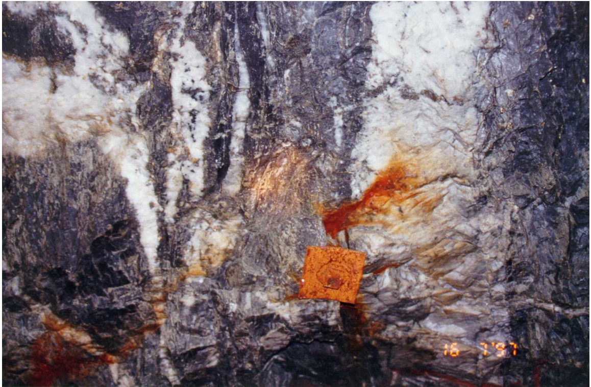
Photo 5. Example of the M1 Vein showing a series of quartz veins and altered mafic volcanic wall rocks. Chip sampling returned 17.6 g/t Au / 0.7m. Rock bolt for scale. -150m Level, Marlhill Mine. Photo courtesy of Pentland Firth Ventures Ltd.
