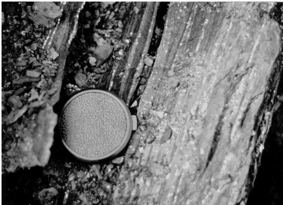
Photo 4. Dark grey coloured carbonaceous greywacke containing disseminated euhedral pyrite along bedding planes. Looking east, 2 Bench, Owl Creek open pit. Diameter of lens cap is approx. 5 cm. Photo provided courtesy of Dan Brisbin.
