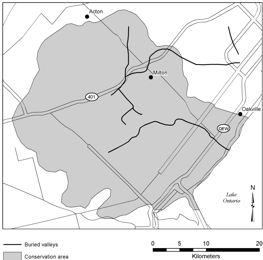
Figure 32.2. Locations of interpreted buried bedrock valleys in the Halton region watershed ( modified after Holysh 1997 ).
