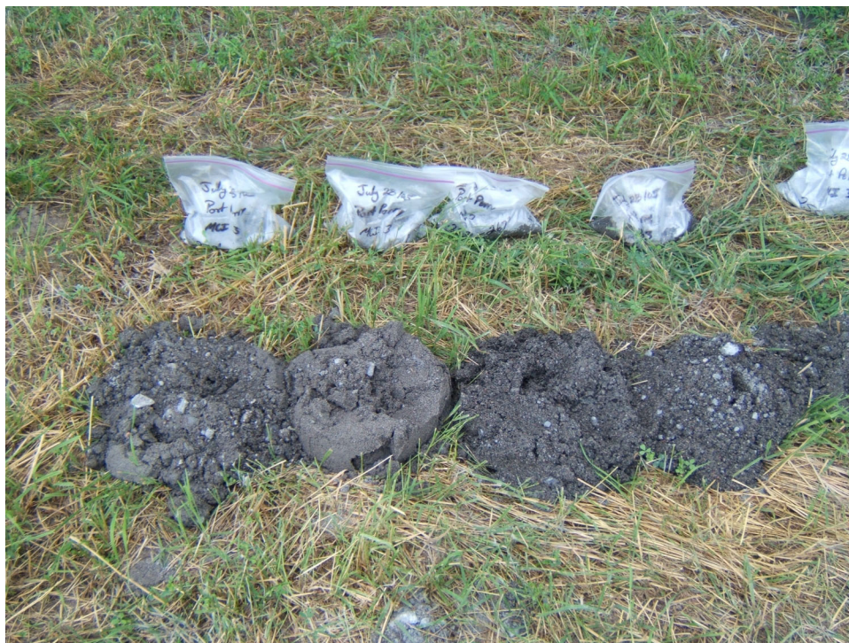
Photo 30.1. Samples obtained from the dual air rotary drilling of borehole CAMC/YPDT-PP-4 th Line near Port Perry.
