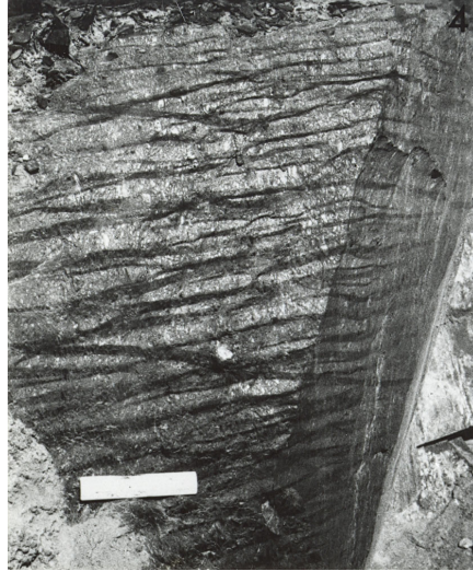
Photo 9.3. Closely spaced kink bands in the Onaping Formation as exposed on the Gordon Lake Road. Ruler is 16 cm long. For location of the kink bands, see Figure 9.1.
