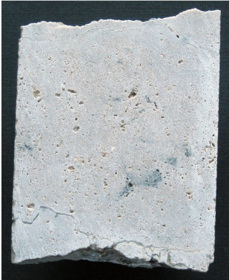
Photo 2. Photograph of a drill-core sample showing a typical example of the Goat Island Formation. The diameter of the core is 6.1 cm (left to right).
