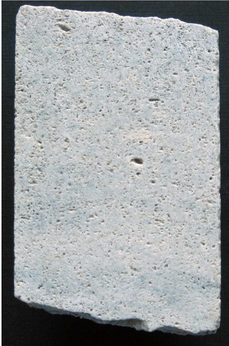
Photo 3. Photograph of a drill-core sample showing a typical example of the Gasport Formation. The diameter of the core is 6.1 cm (left to right).
