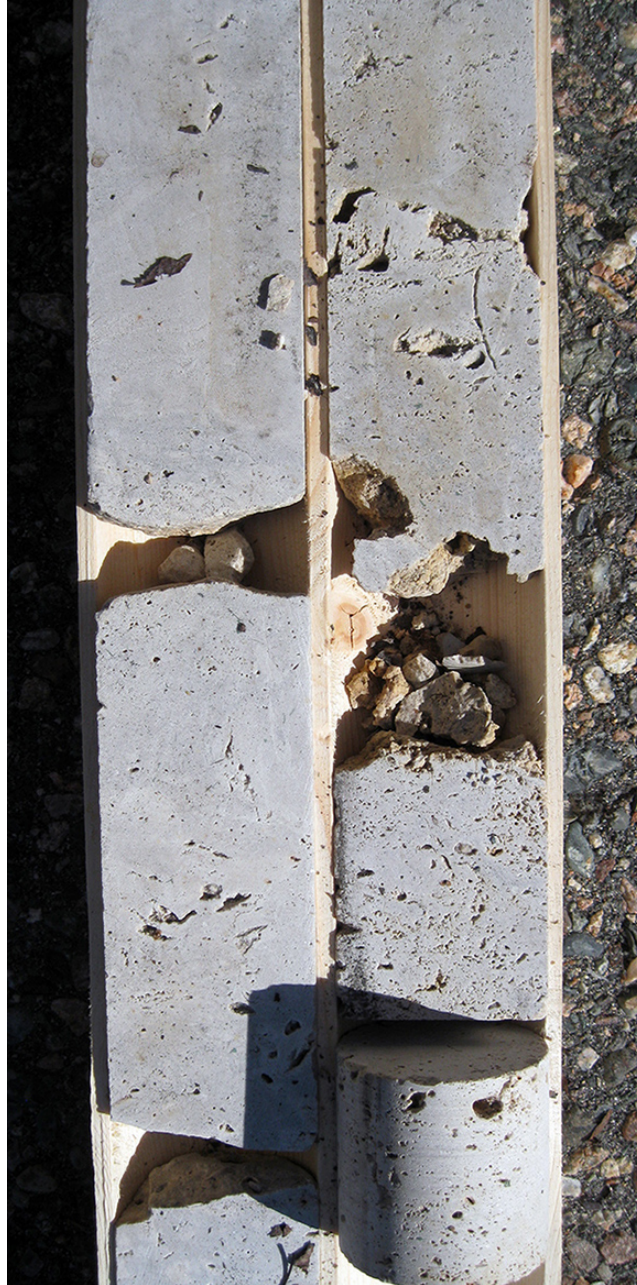
Photo 4. Photograph showing the Guelph Formation from the Elora drill core (aggregate test site 21: depth 20.15 to 21.25 m). The diameter of the core is 7.5 cm (left to right).
