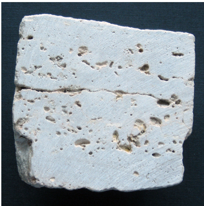
Photo 1. Photograph of a drill-core sample showing a typical example of the Guelph Formation. The diameter of the core is 7.5 cm (left to right).
