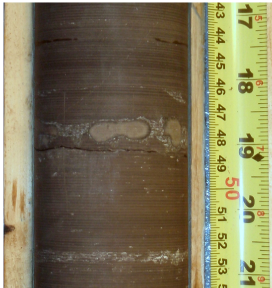
Photo 2. The phosphatic nodule bed corresponds to the contact between the Rouge River (above) and the Collingwood (below) members at a depth of 476.90 m. The top of the core corresponds to the top of the photo.
