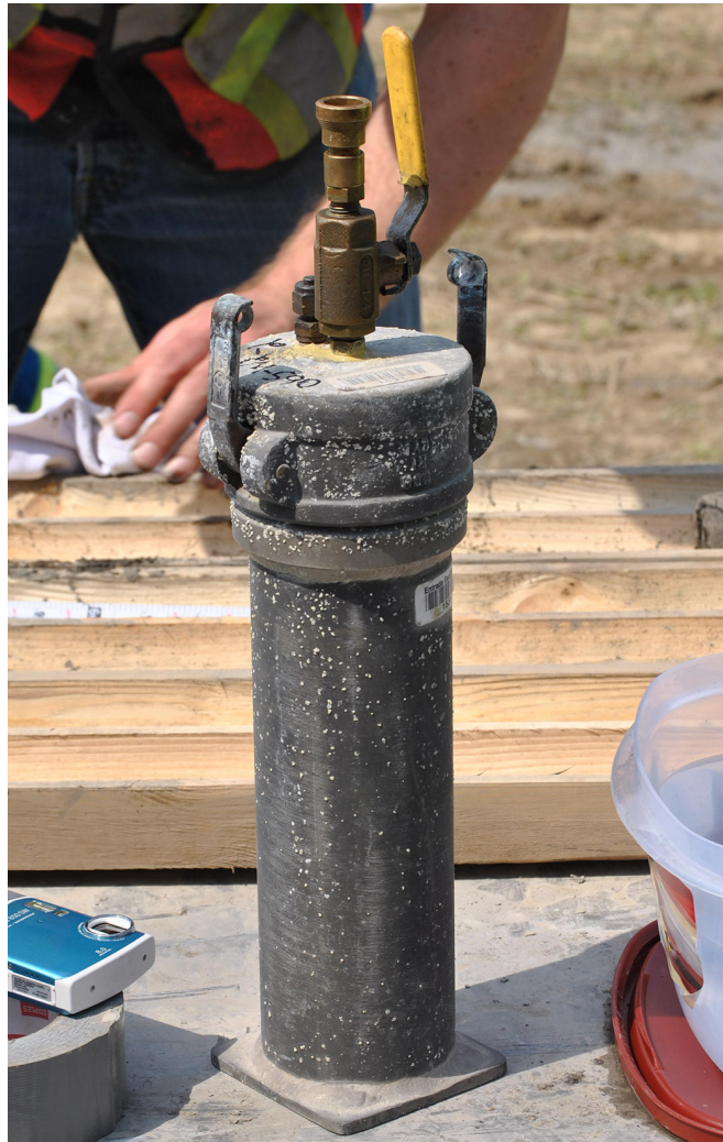
Photo 1. Gas canister used to collect core samples for gas desorption analyses and adsorption isotherms. The height of the canister is approximately 30 cm.
