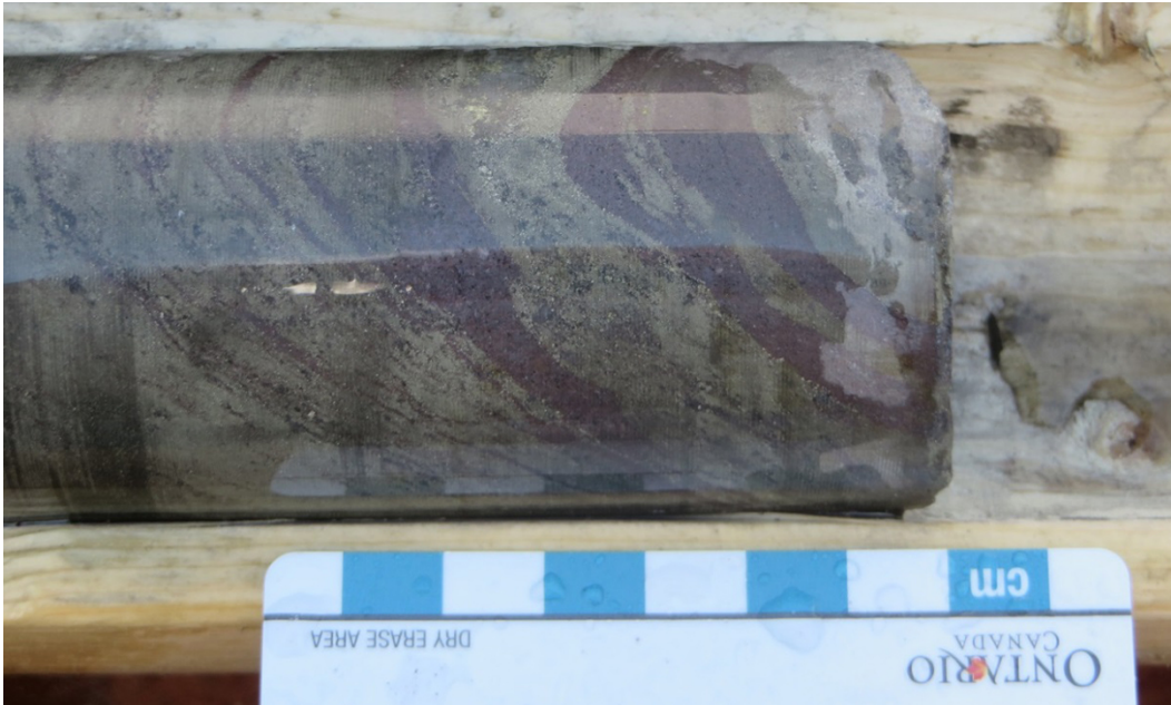
Photo 3. South Bay Mine massive sulphide core from DDH 007. Brown mineral is sphalerite; brass-coloured minerals are predominantly pyrite.
