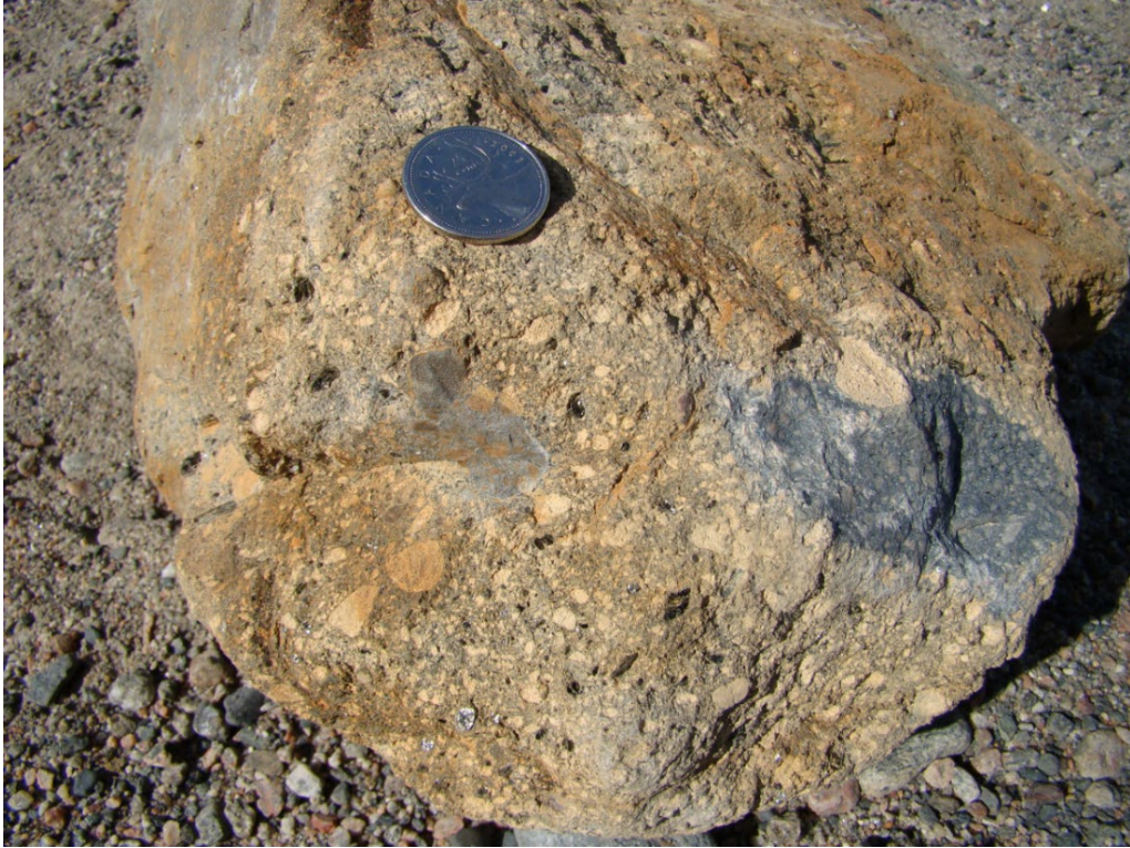
Photo 5. Close-up view of kimberlite boulder 11-CG-068-K, showing dark phlogopite flakes and whitish, oval calcite clasts. Coin 2.3 cm diameter.
