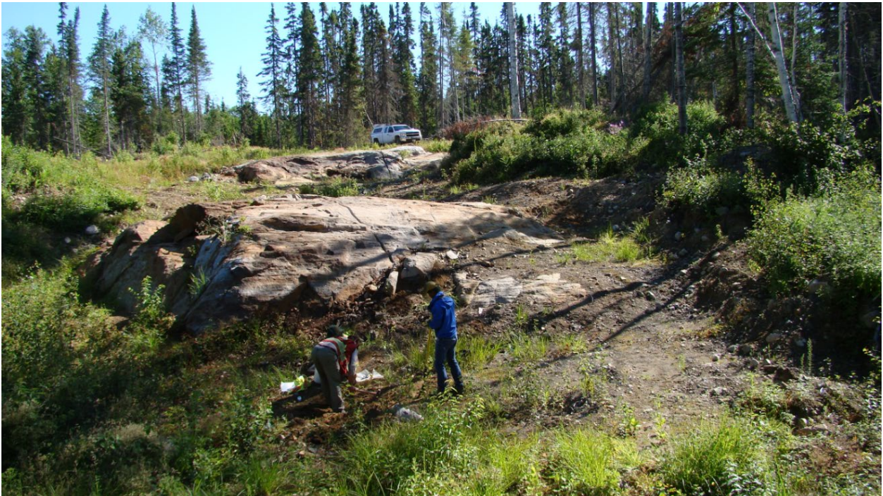
Photo 3. Sampling till immediately down ice of the discovery bedrock outcrop on the Borden Lake gold property. The samples collected at this site all contain elevated gold grain counts.
