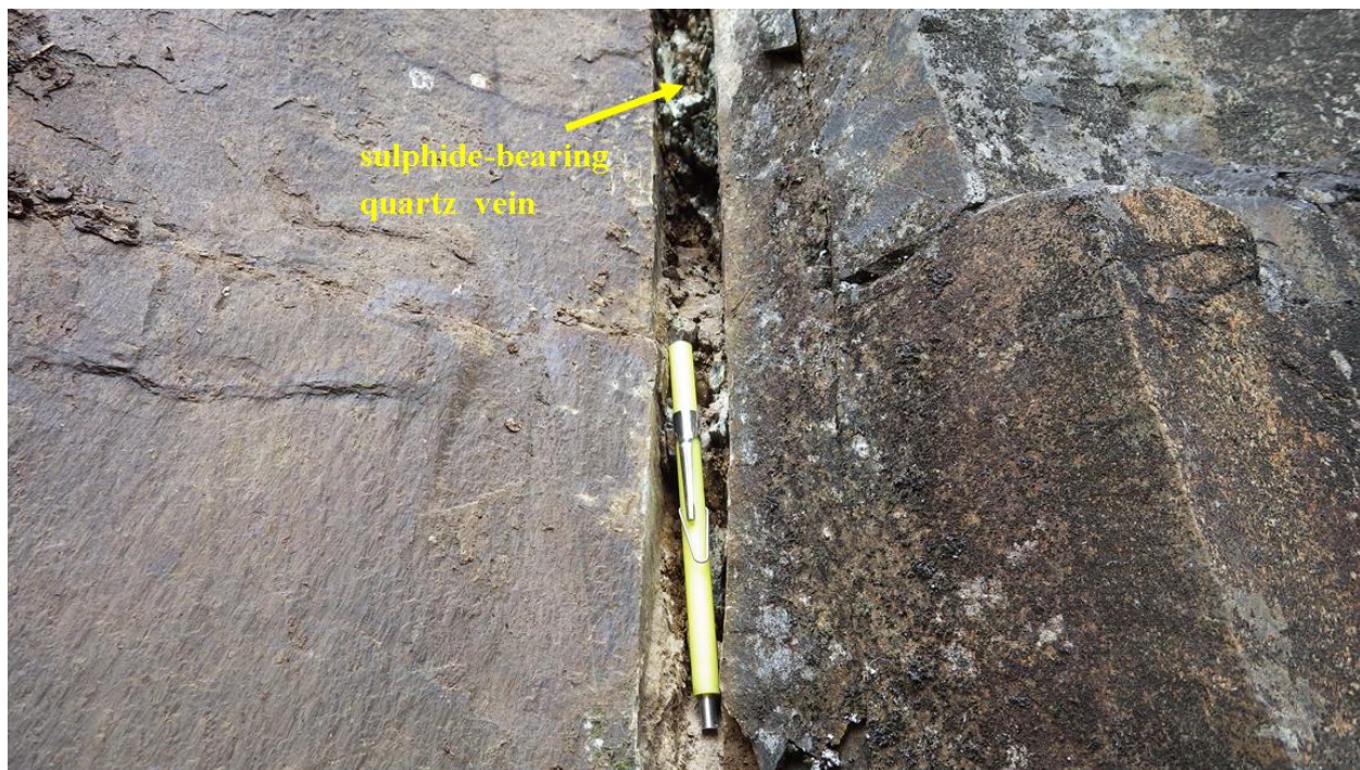
Photo 1. North face of trench with 3 cm wide near-parallel, pyrite-chalcopyrite-bearing quartz vein at UTM 594296E 5338846N; looking north. Magnet pen is 12.3 cm long.
