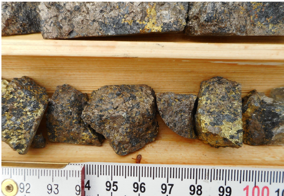
Photo 5. Massive sulphide intersection with pyrrhotite (brown), chalcopyrite (yellow) and sphalerite (dark grey) in Adroit Resources Inc. diamond-drill hole SC-20 (2007), Simon copper prospect, Lyndoch Township; from a section averaging 1.28% Cu and 0.38% Zn over 7.25 m (Parry and Kleinboeck 2007); photo by P.S. LeBaron, August 2019.
