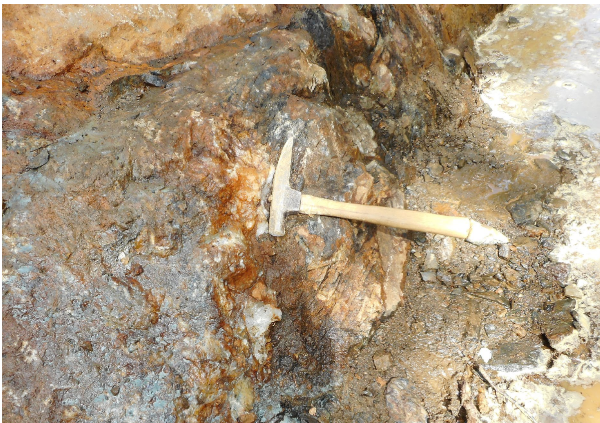
Photo 3. Shallow-dipping, extensional quartz vein in siliceous iron formation, Waring Creek gold prospect (UTM 314638E 4968307N); hammer is resting on the plane of the quartz vein, vein is about 15 cm thick. Photo by P.S. LeBaron.
