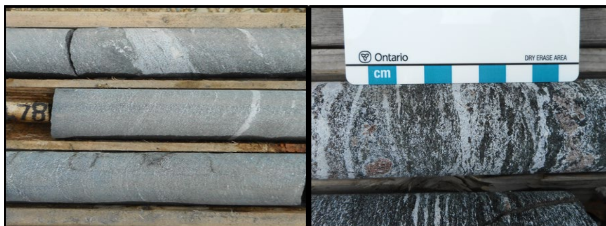
Photo 1. Left: Fine-grained, weakly foliated amphibolite and right: strongly foliated, garnetiferous amphibolite gneiss in Adroit Resources Inc. diamond-drill hole SC-18 (2007), Simon copper prospect; core diameter 4 cm; photos by P.S. LeBaron, 2019.
