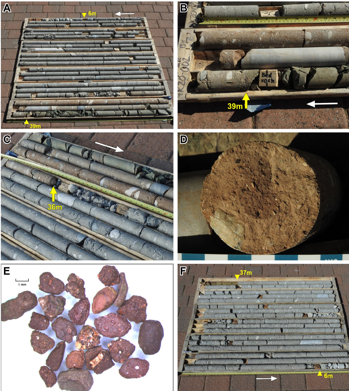
Photo 15.2. Photos from drill-cores HK20-002 (A to E) and HK20-004 (F). White arrows indicate up-core direction. Core boxes are 1.5 m long. A) Drill-core HK20-002, consisting of a thick grey till (unit II) underlain by a red till up to 3 m thick (unit I). The uppermost 6 m of the core has poor recovery (above the yellow triangle). The contact between the red till and underlying greenish shale bedrock is at 39 m depth (yellow triangle). B) Close-up view of the sharp contact between the red till and greenish shale bedrock (yellow arrow). Note the presence of surface mud coating renders the red till to appear less reddish in colour. C) The sharp upper contact of the red till (yellow arrow) at 36 m depth. The overlying grey till has a poor core recovery at the interval immediately above this contact (36–33 m depth). D) Enlarged view of the red till (unit I) in a core segment at 36.1 m depth, which is a calcareous, highly compact, structureless silty diamiction. The light-toned, large pebble on the lower left is a Paleozoic limestone. Scale in centimetres. E) Red to reddish brown arkosic sandstone clasts in the red till, which were picked from 2 to 0.125 mm fraction of a washed sample. F) Drill-core HK20-004, consisting almost entirely of the grey till (unit II). It has poor core recovery above 6 m depth (yellow triangle). Its sharp contact with the greenish brown shale bedrock is at 37 m depth (yellow triangle). Refer to Figure 15.1 for the lithostratigraphic units mentioned.
