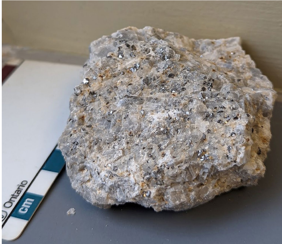
Photo 8. Mineralized graphitic calcite marble from the K9 property. Note the shiny, silver and rounded graphite flakes. Sample is approximately 7 cm across.
