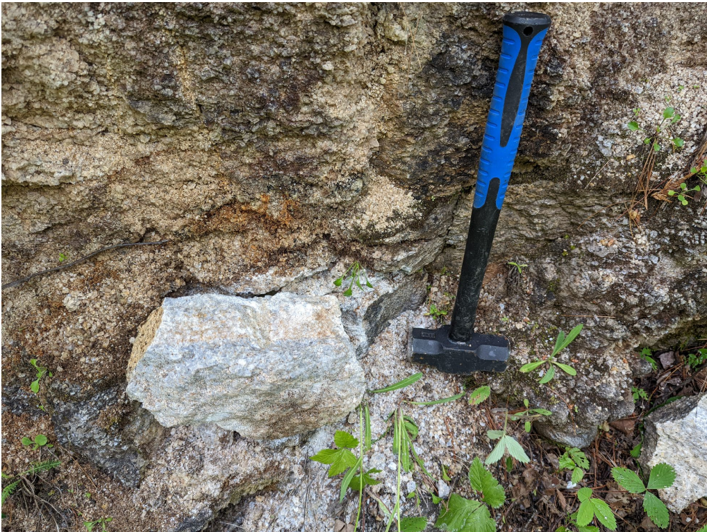
Photo 7. Blue graphitic calcite marble from the K9 property. Note millimetre-scale graphite flakes. Hammer, for scale, is 42 cm long.
