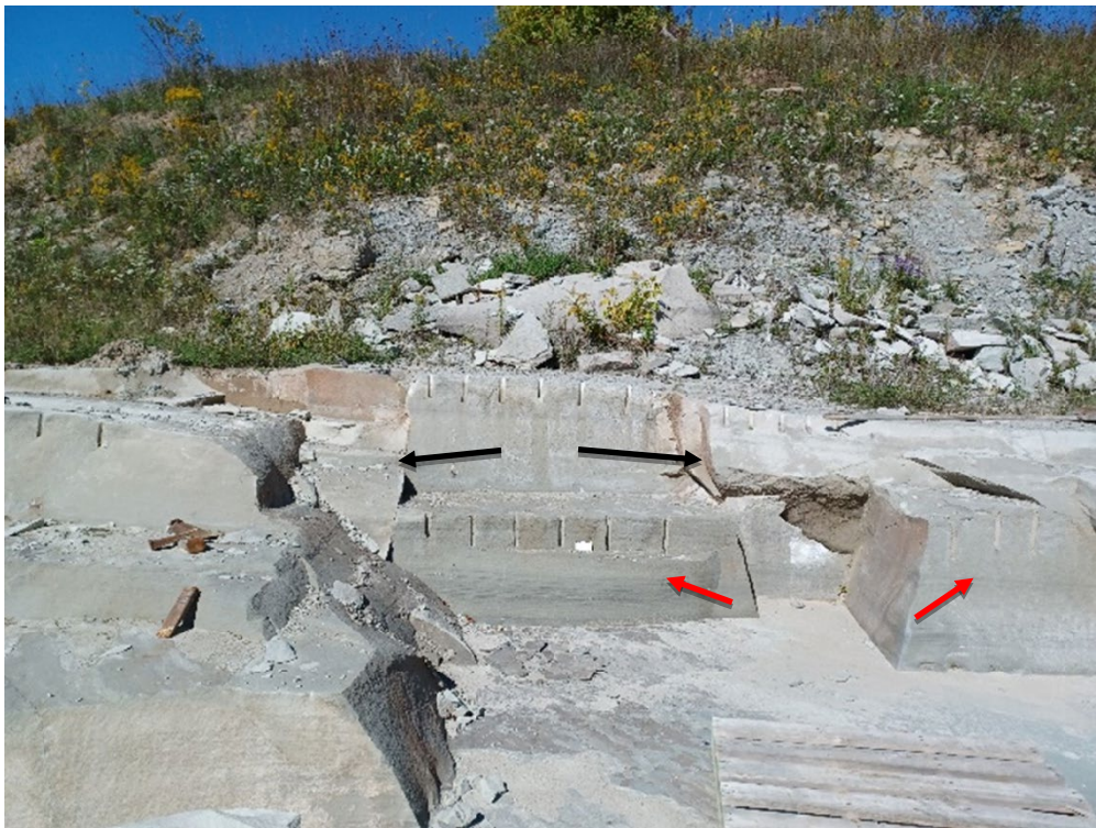
Photo 5. Joints and laminations in within the Rice and McHarg Quarry Whirlpool Formation sandstone. The black arrows point to one of the 2 joint sets and the red arrows point to the laminations.
