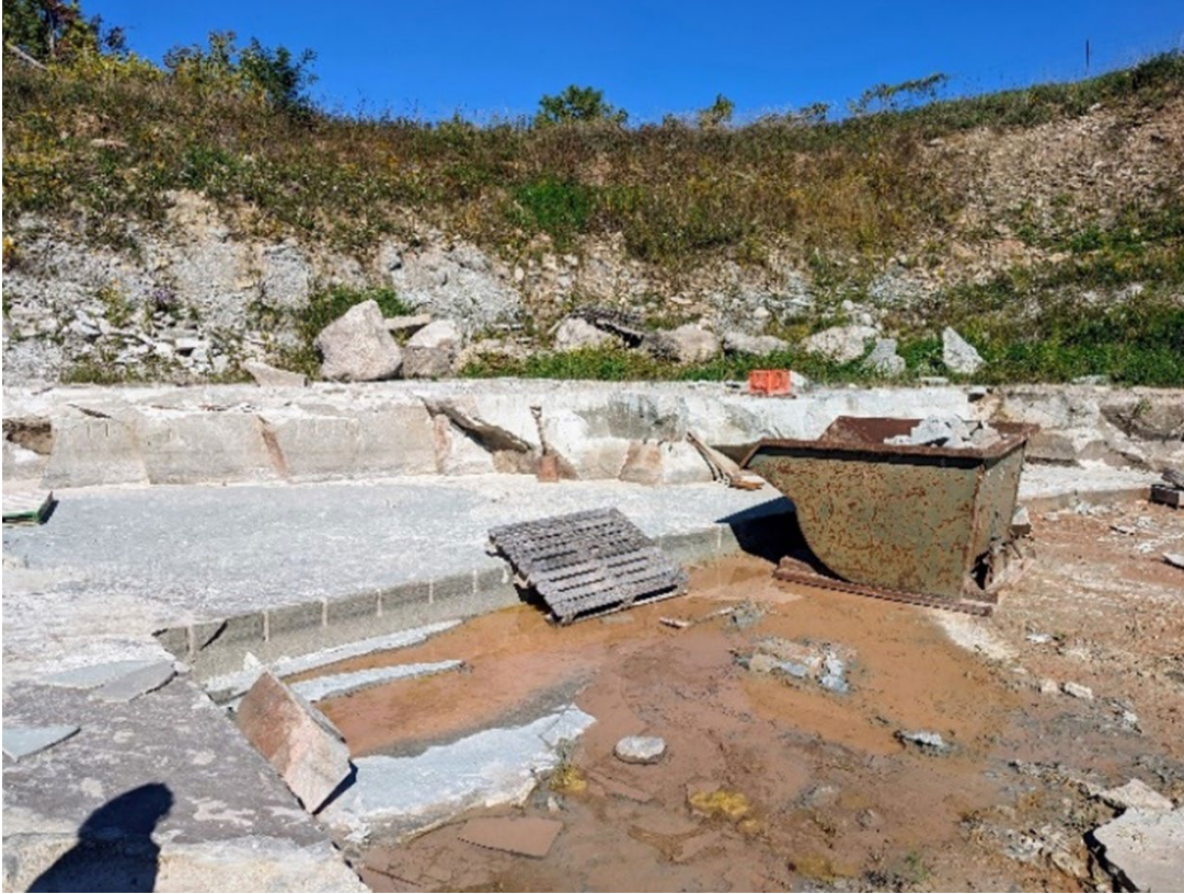
Photo 1. Rice and McHarg Quarry Whirlpool Formation sandstone overlain by 2 m of shale and 2 m of clay overburden.
