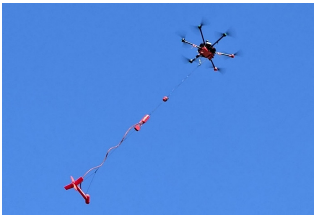
Figure 28. Drone with a magnetic sensor in tow (photo by Matt Krukowski).
