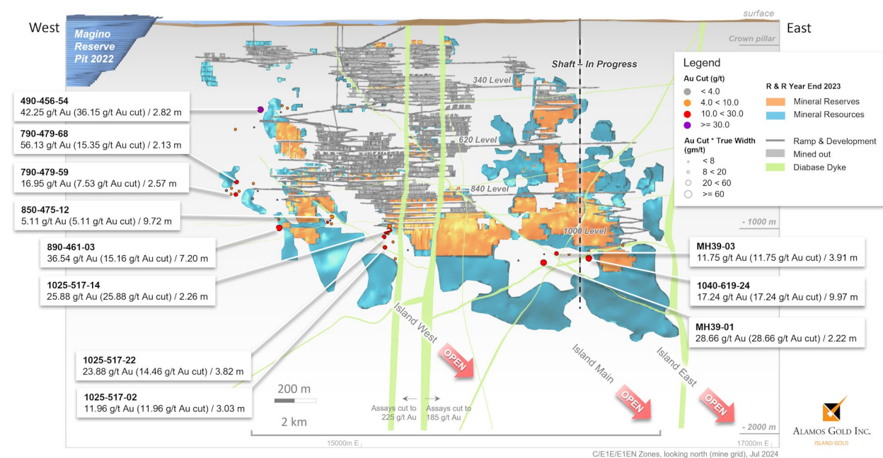
Figure 4. Underground exploration drilling activity at the Island Gold Mine. Longitudinal section through C- and E1E-Zones showing underground exploration drilling results (from Alamos Gold Inc., news release, July 23, 2024).
