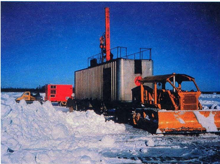
Holes are drilled into lake bottoms from winter ice to test indications that mineral deposits might lie under the lakes
