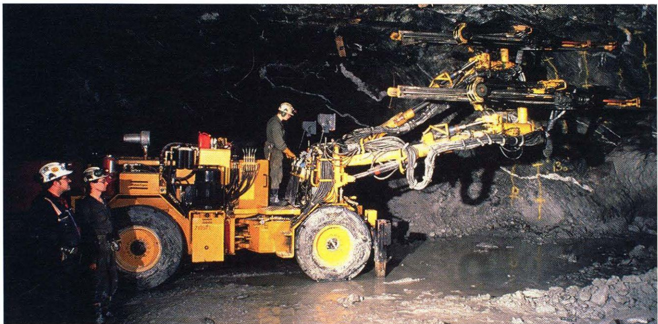
Machines like this are used to drill holes for explosives in underground mines
