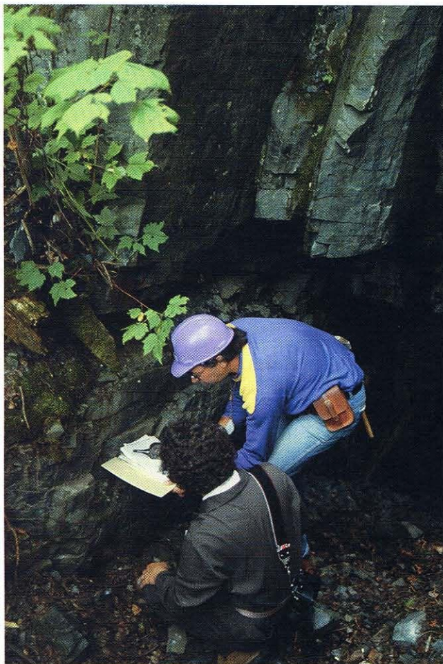
The contact between Nipissing diabase (upper), and Cobalt Group rocks (lower) is the site of many of the silver deposits in the Cobalt area
