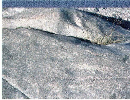
PHOTO 63: This granite at Rossport Provincial Campground has coarse grains of feldspar embedded in a finer-grained matrix of other feldspar, quartz, and mica. Rock like this can be used to make attractive building stone.
