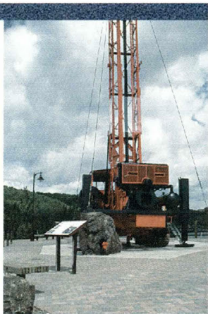
PHOTO 100: The large drill at Wawa's waterfront park is one of the drills that was used to prepare blastholes at Wawa's open pit iron mines.
