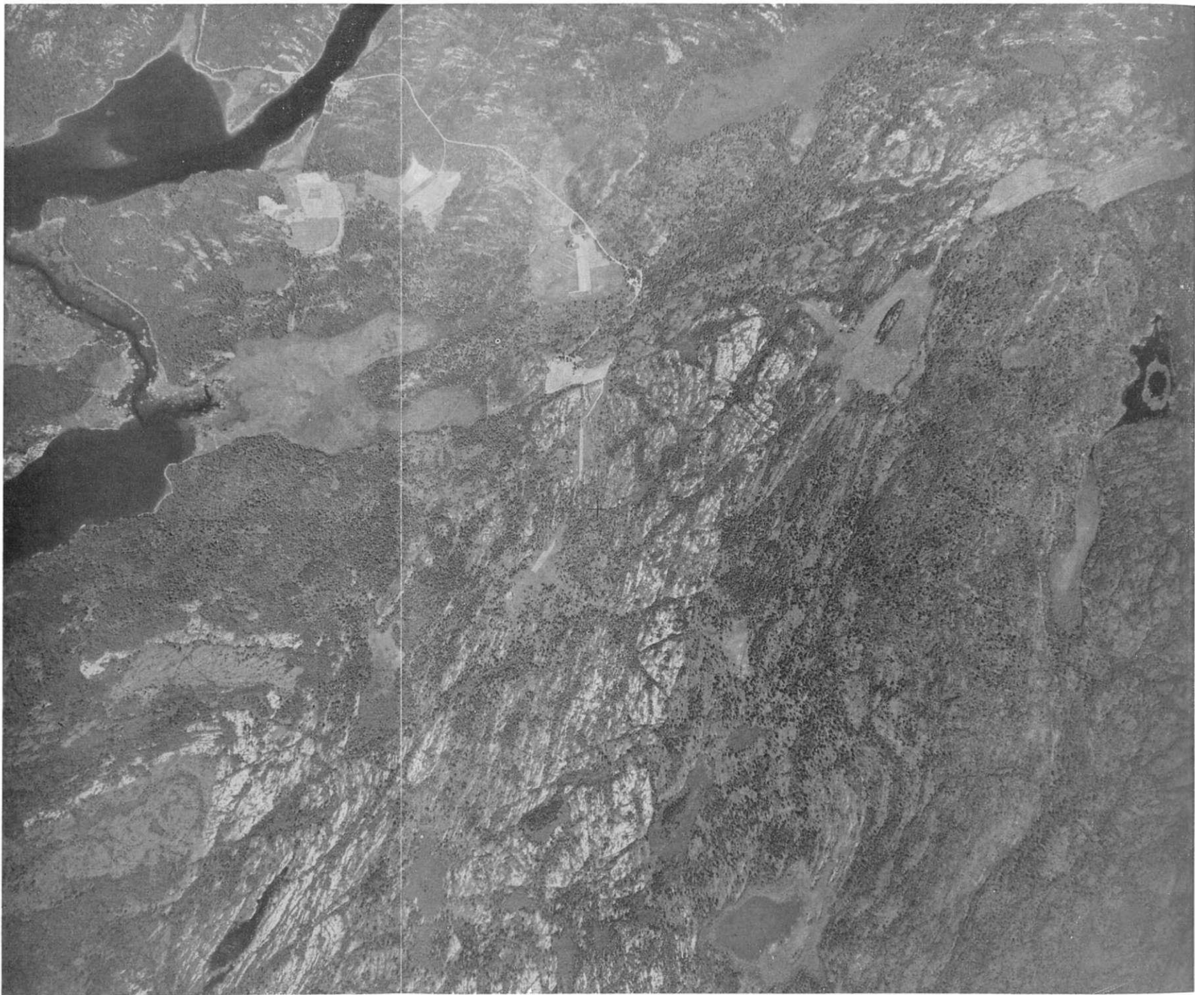
An air photograph of part of Lorne township, west of Margaret Lake. The Red Pine syncline is evident in the bottom left corner of the photograph. Note the differences in appearance of quartzite (white), argillaceous sediments (banded grey) and gabbro (elephant hide appearance). (Air photo 46-164/15-32, courtesy Ont. Dept. Lands and Forests.)
