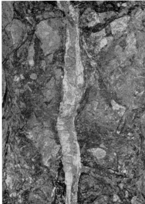
Photo 5 — Vein 30, Langis No. 3 shaft workings; rich silver-cobalt vein about 6 inches wide in Gowganda conglomerate. (Photo courtesy of J. E. Jerome.)
