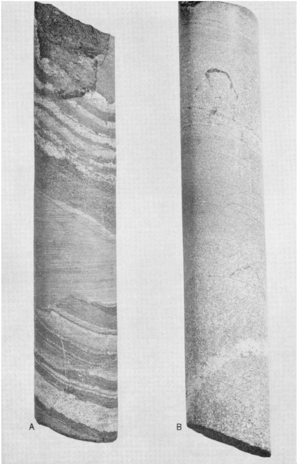
Photo 9 — Core A: Cut-and-fill structure in banded iron formation. Core B: Graded bedding in quartzite. Both structures appear useful as top indicators. (Diam. of core is 1\frac{1}{4} in.).
