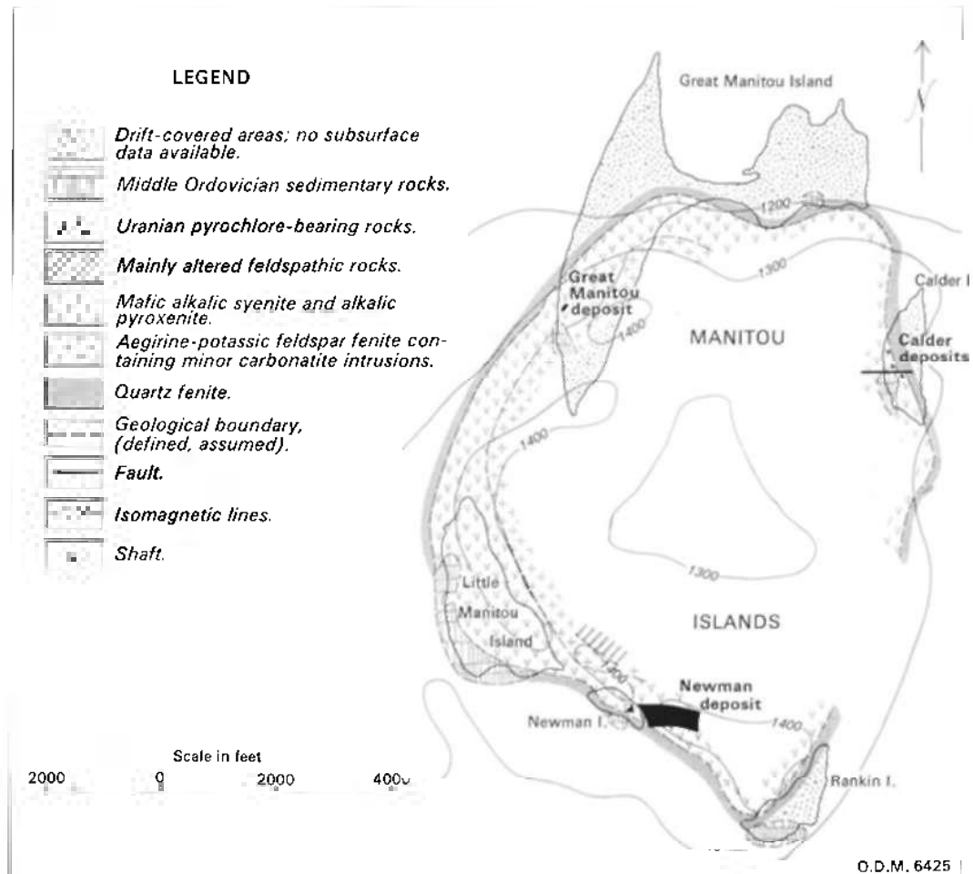
Figure 6—Sketch map showing the major geological features and mineral deposits of the Manitou Islands Complex (modified after Rowe 1958, Figure 14).
