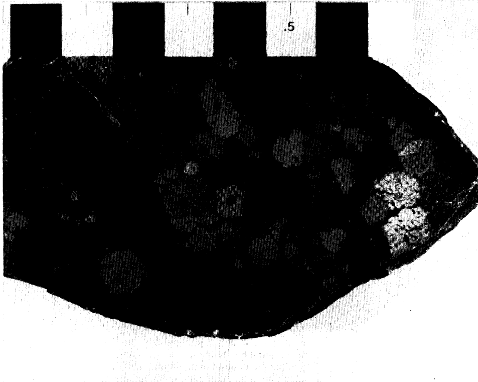
Photo 12—Massive ore, Shebandowan Mine. Pyrrhotite-pentlandite matrix with nodular phenocrysts of pyrite partly surrounded by chalcopyrite. Fragmented inclusion of serpentinized peridotite visible in bottom centre of photo.
