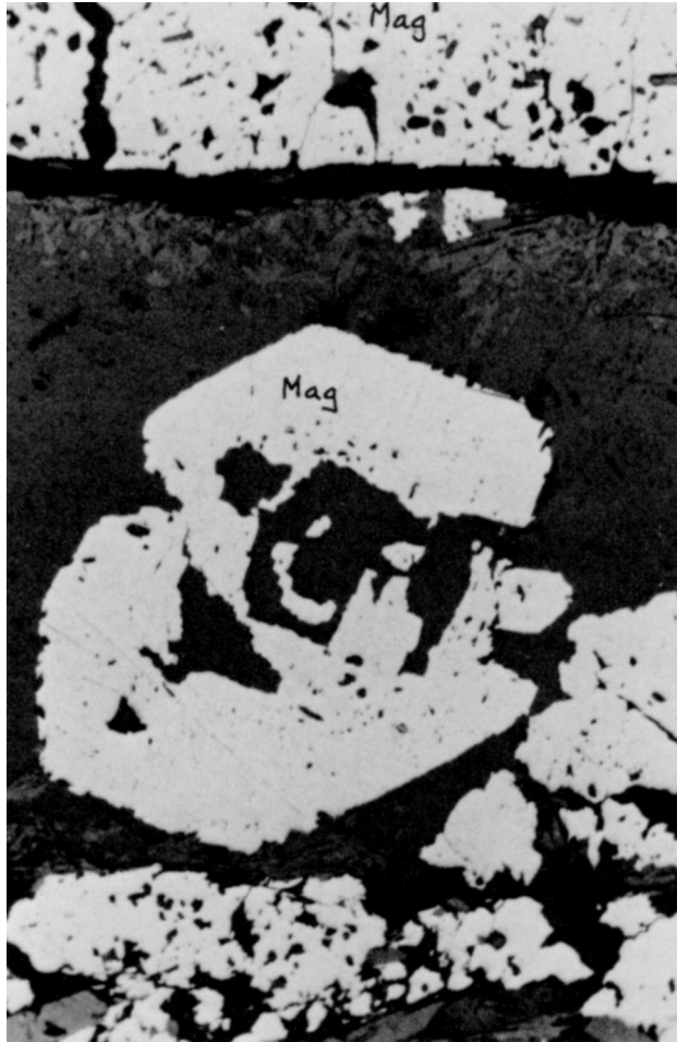
Photo 12—Photomicrograph of magnetite mineralization, Bardswich Lake magnetite deposit, Hess Township. 10X Magnification. Note the mineralogical layering with alternating magnetite-rich and gangue-rich layers with skeletal magnetite crystals.
