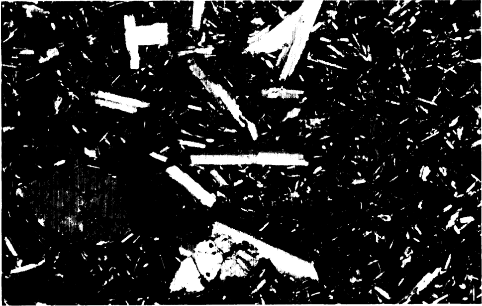
Photo 13—Aphanitic, porphyritic olivine diabase. Plagioclase laths and little olivine in an almost opaque groundmass. Westshore of Portage Bay. Scale 0.4 mm. Crossed polarizers.
